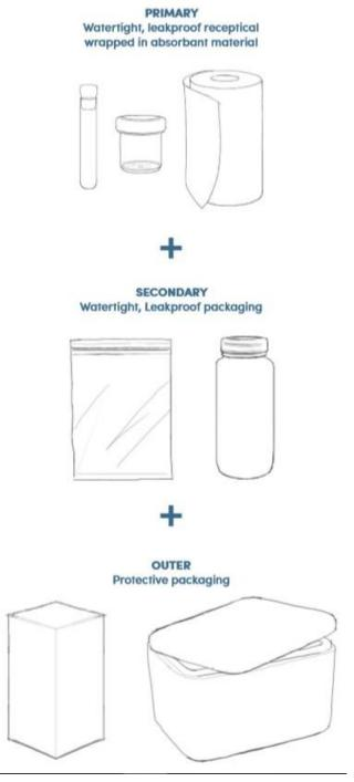
Figure 4: examples of basic triple packaging materials
